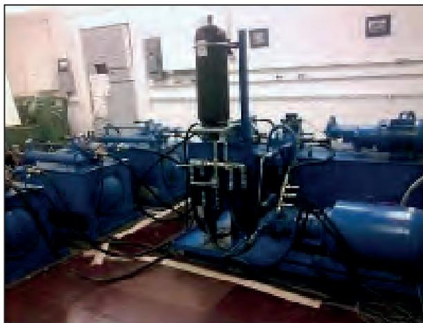
Figure 1: Augmented Earthmoving Vehicle Powertrain Simulator
