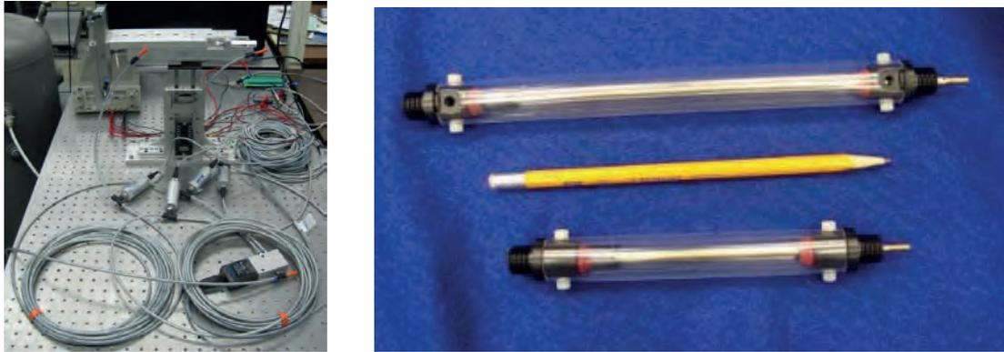
Figure 1-2: Line dynamics control testbed. This experimental setup consists of a pneumatic cylinder connected to a computer-controlled valve via long transmission lines. The figure on the right shows the MRI compatible pneumatic cylinders currently under investigation.
