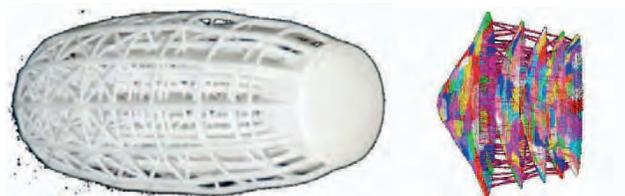
Figure 4: Preliminary automated generation of 3-D multi-functional structure. (Left) Concept model, fabricated on MSOE-RPC’s SLS. (Right) Preliminary database-driven algorithm output.
