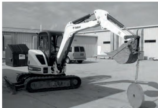
Figure 2: Power management fuel test setup
