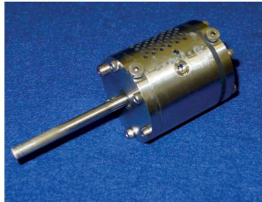
Figure 1: Version V1 vane motor prototype.
