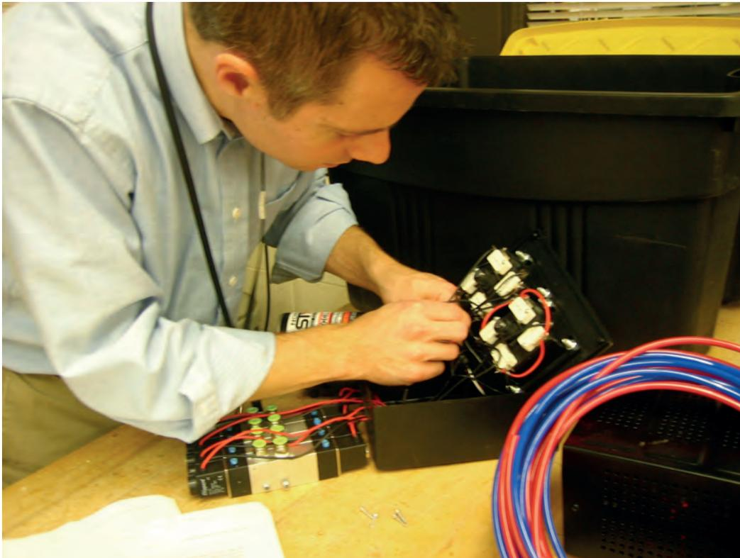
*A Project Lead The Way Teacher, also an RET at Purdue University, works on the Portable Water Hydraulics Demonstrator under the guidance of Professor John Lumkes.*
