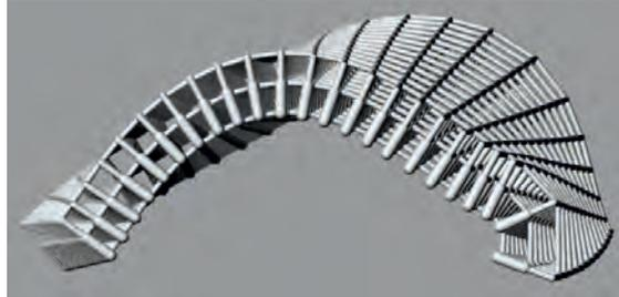
Figure 5: Automated conformal structure generation using the Cube lattice unit cell. As shown, the struts are sized independently in each of the orthogonal directions, at each layer.
