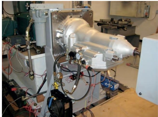
Figure 5: FTI Hydro-Mechanical Transmission on the dynamometer test-stand at the FTI site.
