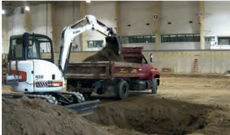
Displacement controlled excavator uses 40% less fuel!
