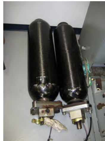
Integrated HMT on a dynamometer test-stand (left) and hydraulic accumulators to be used as energy storage elements.
