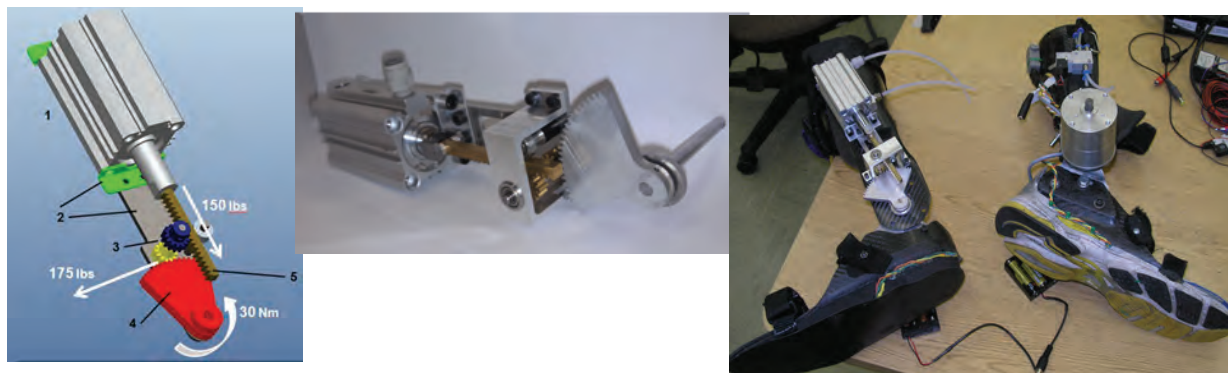
Figure 3. CAD and physical models of design which used an off-the-shelf linear actuator with sector gear to create torque about the ankle axis by AY12-13 team. Right panel: comparison of linear design with commercially available pneumatic rotary actuator.
