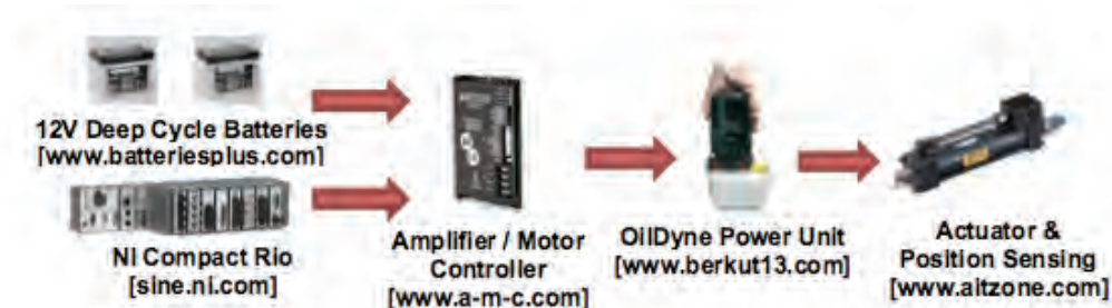
Figure 1: Power and Actuation for Each Degree of Freedom Using Electro-Hydraulic Pump Control.
