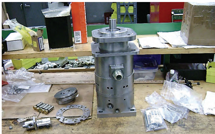
Figure 1: Picture of partially constructed discrete piston pump/motor prototype
