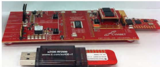
a) Off-the shelf harvester power conditioning circuit and wireless transmitter/receiver
