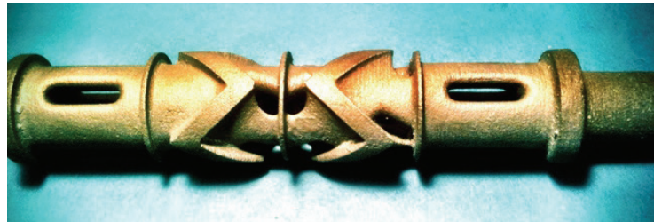
Figure 5: Cast 4-way rotary valve spool prototype from MSOE
