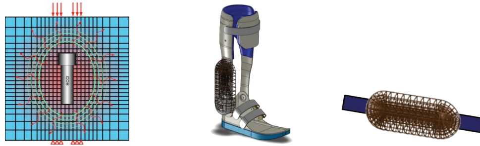
Figure 1: (Left) Concept of the mini-HCCI engine with an integrated noise-filtering and heat-dissipating structure. The structure also bears mechanical loads, so it can be integrated into the structure of the Test Bed 6 PPAFO. (Center) Conceptual model of the integration into the PPAFO. (Right) Conceptual model of a belt-worn structure that contains the engine's temperature, while also protecting the wearer and reducing noise.
