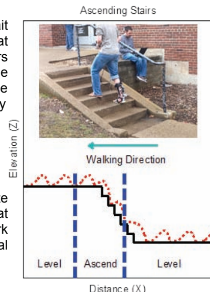
Figure 2: Stair ascending gait mode recognition. Real-time 3D PPAFO position was tracked using a 6DOF IMU at the toe.
