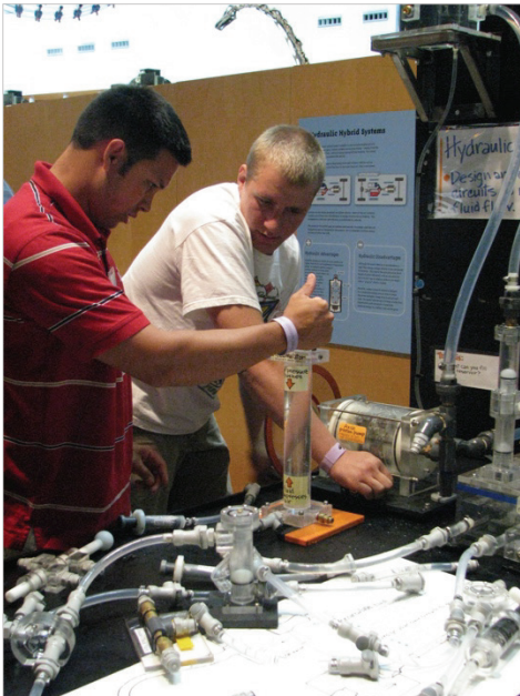
Figure 3: Hydraulic variable torque transmission with accumulator-based energy storage.
