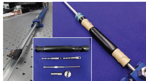
Figure 7: Experimental Prototype of the Distributed Piston Accumulator loaded into a hydraulic cylinder (piston rod provided only for measurement of displacement). Elastomeric member shown with cylinder casing removed. Inset shows clamping schemes.
