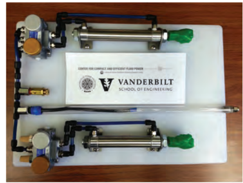
Figure 5: Pneumatic strain energy accumulator implemented on interactive breadboard demonstrator
