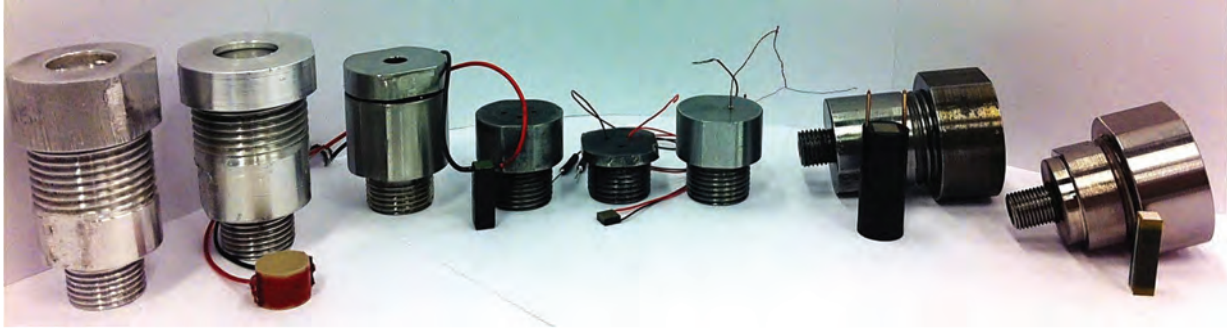
Figure 3. HPEH prototypes with threaded connector for attachment to fluid hydraulic systems; successive generations, left to right to the center of the picture, designed for smaller piezoelectric element and more compact packaging. Later generations, from center of the picture to the right side of the picture, designed for specific piezoelectric performance assessment and alternative seal designs (center), and HPEH integration with existing commercial hydraulic sensor housings (right two prototypes).
