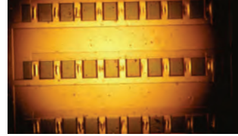
Deformation of piezobenders (visible as warping of center of beams).
