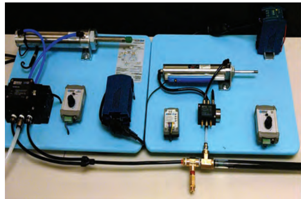
Figure 6: Pneumatic strain energy accumulator implemented on industry partner automated breadboard demonstrator
