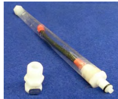
Figure 4: Quick disconnect pneumatic strain energy accumulator
