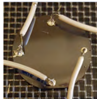
(d) Assembled Prototype on Orifice Plate Side with Lead Wires*
