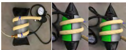
Figure 5: Experimental setup using FREE actuator, 3D printed shells and air bladder and cylinder
