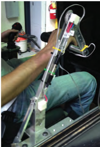
A kinematically similar interface controls the vertical motion of an excavator arm. The cab swing rotation is still controlled by a joystick.
