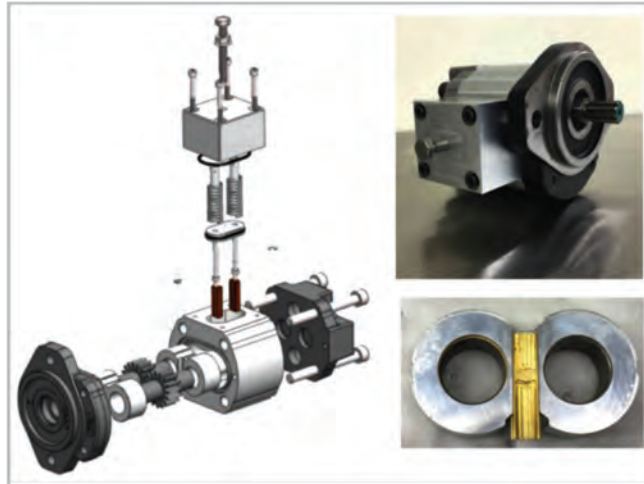
Exploded view of the proposed variable displacement external gear machine as well as the prototype produced as an outcome of project 1F.1
